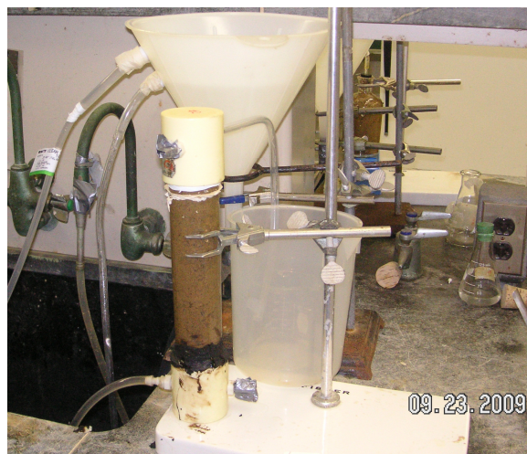
Figure 1. Setup of a soil column used for the sodium injection experiments.
